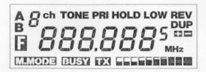
The LCD Screen displays many of the functions selected by the keys on the front panel. These functions are shown on the Screen Drawing shown above.
