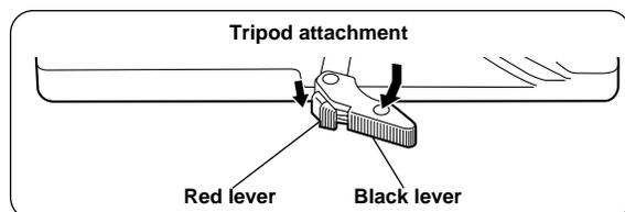
While pushing down the red lever, move the black lever in the direction of the arrow and slide the unit toward the back to remove it.
