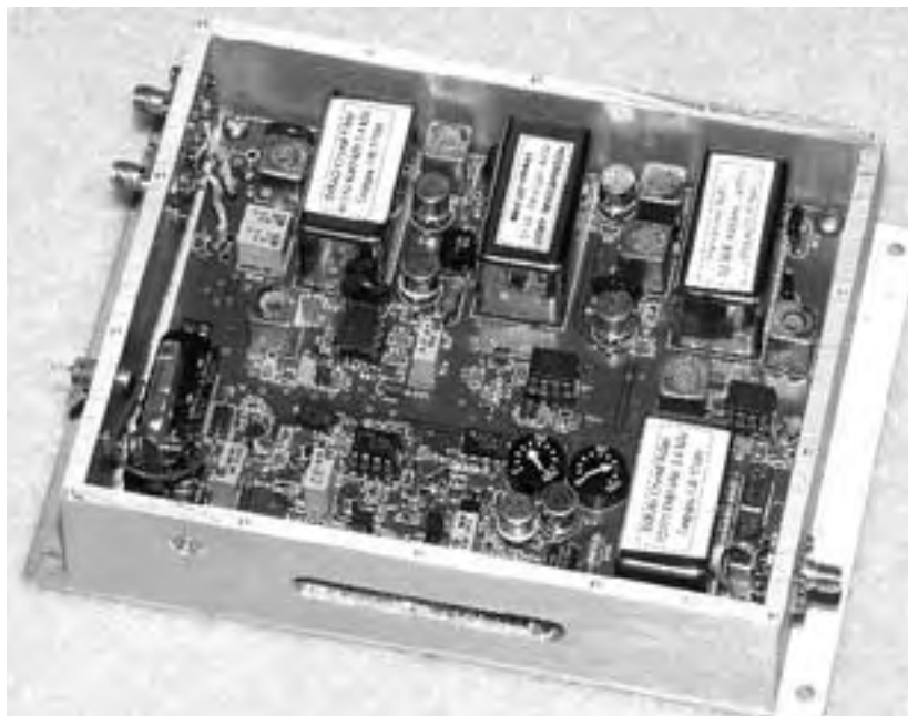
Figure 26 — Actual implementation of the IF9RX assembly. A specific double side ground plane stitched - plated through layout is used to maximize isolation between input circuits and output circuits in order to prevent oscillation in this very high gain (100 dB) assembly. All Quartz filters on the assembly have been expressly manufactured for the Star-10 by International Filter Company.
