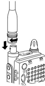
Fit the base of the antenna over the projections on the connector, press downward and turn clockwise. Check the antenna is securely attached.
