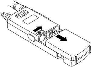
Slide the battery pack lock on the case to the right and pull the case downward to detach.
