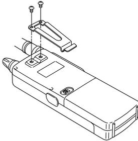
Screw the belt clip onto the rear panel (screws x 2). Check the clip is securely attached before use.
