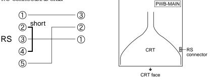
2. In the adjustmentmenu, select "Function" on the Main Menu and then select "Language" on the Sub-Menu. Follow the flow chartbelow and you are in the Factory Mode. Turn OFF the PowerSwitch to exit.
