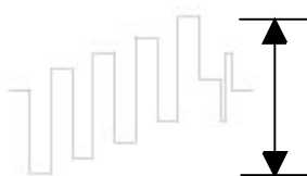
Fig. 20 Signal Pb Pin 3 of Connector P0YU ; 1Vpp
