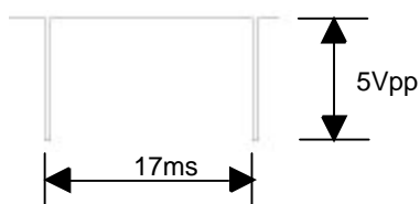
Fig. 18 Vertical Sync Signals TP5854
