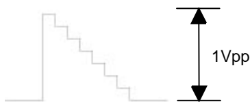
Fig. 14 Signal RGB Pins 1, 3, and 5 of connector P0PC
