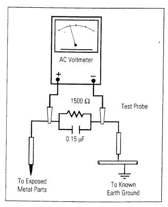
Figure 1-1. Leakage Current Test Circuit
