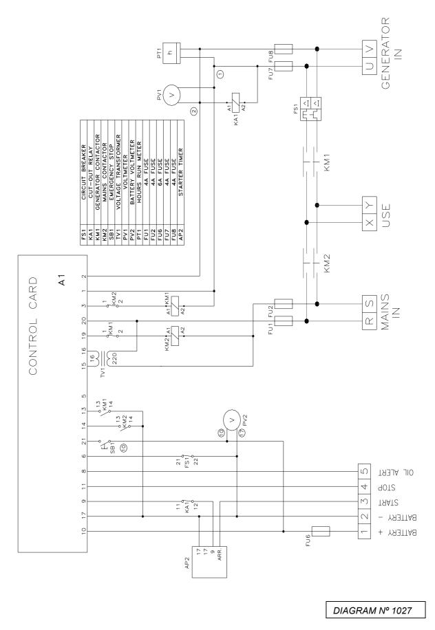
WIRING DIAGRAM PETROL MANUAL 230V.
