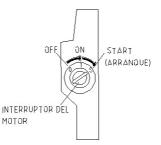
NOTE: Do not use the electric starter for during more than 5 seconds at a time. If the engine does not start up, release the key and wait ten seconds before trying again.
