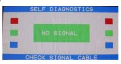
When user does not support the video signal from the cable this dialog will appear about 10 seconds. And then enter the Sleep mode. One special case was in factory mode, the display time length will become 5 seconds for testing the power consumer.
