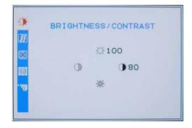
When user press the **Menu** key under none OSD status will trigger this menu appear for detail parameters adjust. This menu will display about 20 seconds if no one press other key, otherwise will refresh display time length.
