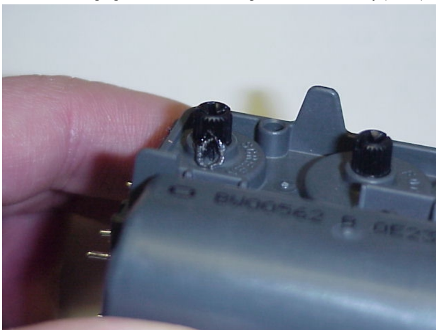
Photo 4. Melting right side of VR knob together with FBT body (Done)
