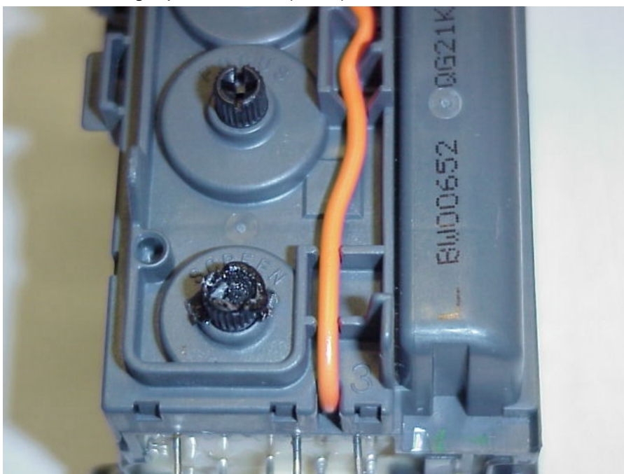
Photo 8. Melting top of VR knob (Done)
