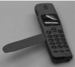
4. Insert the hook release jig (p/n 9-948-370-20) in the gap between upper and lower cosmetic, as indicated in the picture.
