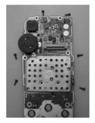
8. Remove 6 screws located on the display side to release the patch antenna.
