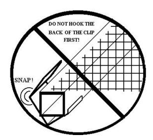
**3. PVC Clip -** The PVC clip is shown above. It is also quite simple. The clip is used to secure the aluminum mesh to the various 1" x 1" box beams. Aluminum stretched mesh is placed on the top surface of the 1" x 1" beam or frame. The mesh should cover most of this surface.
