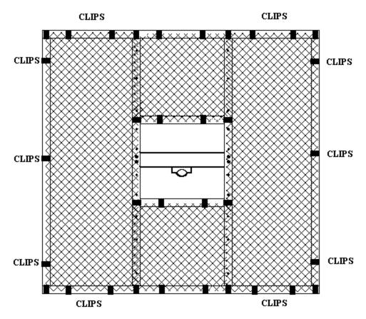
**D.** Now locate the 5/16" stainless steel hex self-tapping screws and washers. Secure both meshes to the box beams, using the screws, washers and nut driver supplied. A total of 20 screws are required.
