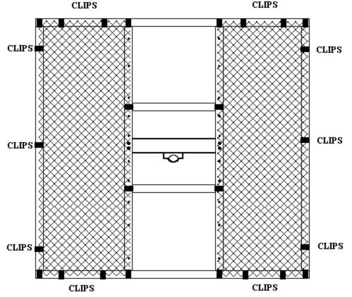
**B.** Locate the two 24" x 23  $\frac{1}{2}$ " mesh pieces. Place them over the 24" x 24" frame. In so doing you will place one edge over the mesh already covering the  $\frac{1}{8}$ " holes. Refer to the figure below.
