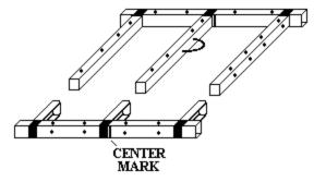
5) Carefully without moving the corners, insert the two 26" tubes into the remaining two prongs of your T frame. Now, carefully line up the other ends of these tubes with the prongs on the other 28" gently slide all three of these tubes over the prongs on the other 28" tube and snug. You have formed a rigid rectangle.
