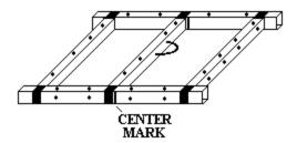
**6)** Slide one corner over the end of each tube. These prongs should point down or away from the screw holes thus creating a little table.
