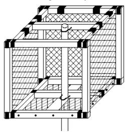
5) Twenty screws attach the two 12" x  $26\frac{1}{2}$ " mesh sections to the frame and complete the mechanical assembly.
