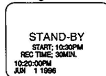
The Palmcorder will start recording at the desired time. When the recording finishes, the Palmcorder will turn off automatically.
