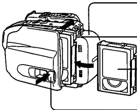
• To remove the cassette, slide the **TAPE EJECT** switch.
