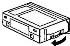
**1** Turn the **Tape Wheel** in the direction of the arrow until there is no slack.
