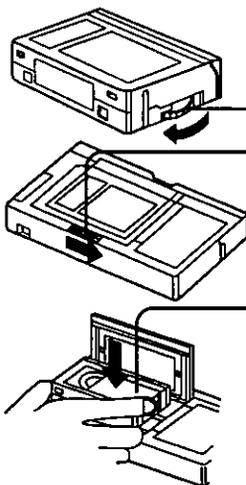
**1** Turn the Tape Wheel on the **VHS** cassette in the direction of the arrow to reduce any slack.
