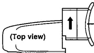
**2** Remove the eyepiece. (Do not twist.)
