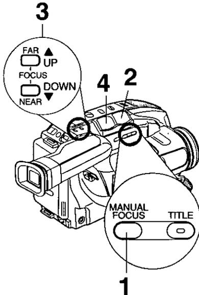
**1** Press **MANUAL FOCUS** so "MF" (Manual Focus) appears in EVF.
