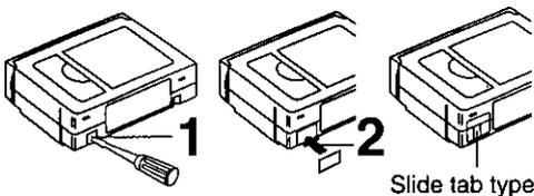
**1** To prevent accidental erasing, **break off tab** with screwdriver. (Or, slide tab open.)
