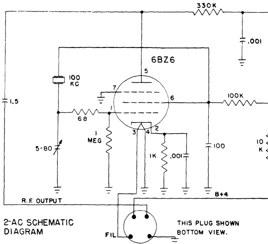
The 100 KC crystal calibrator is an oscillator so designed that it will inject into the receiver a harmonic every 100 KC throughout the receiver's range. This corresponds to the numbered dial divisions on your 2-A or 2-B dial.
